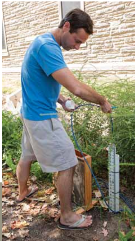
Kevin Flynn MSSE '11 calibrates a pressure transducer, which measures the depth of stored rainfall.
