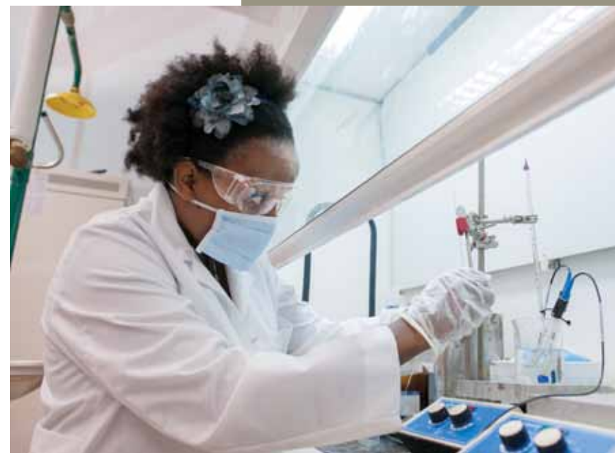
Arlene Wangia MSEE '13 works on the electrodeposition of cadmium telluride solar cells.
