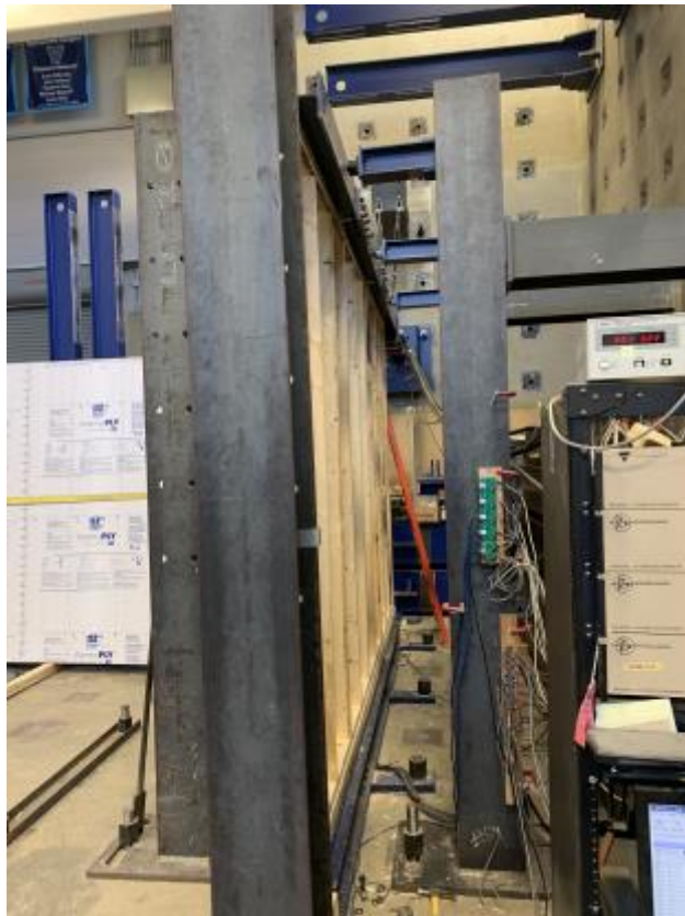
4 - Backside of traditional wall in testing apparatus
