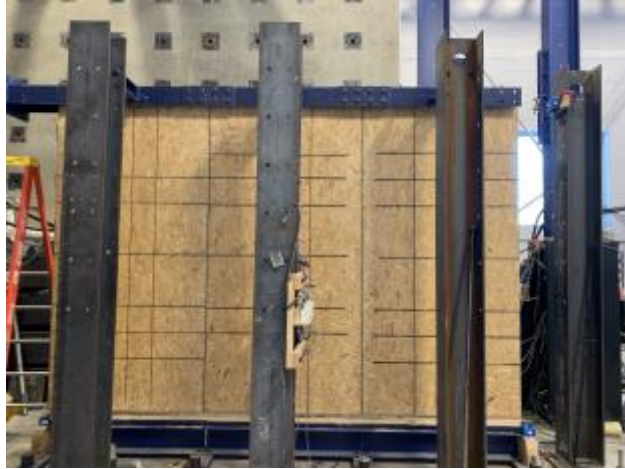
3 - Traditional wall in testing apparatus
