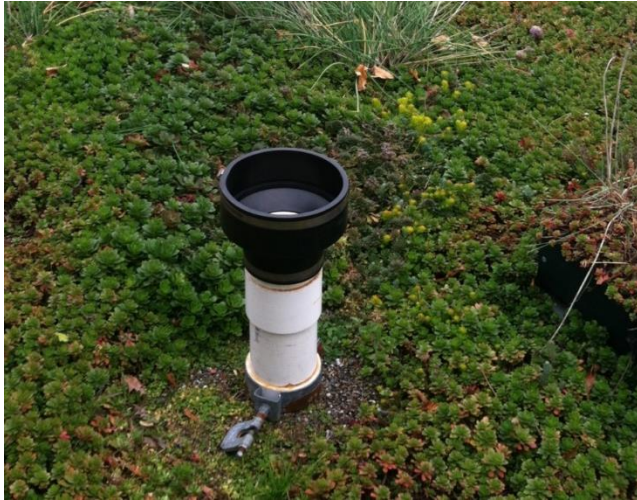
Figure 6: PVC container used to sample precipitation on the green roof
