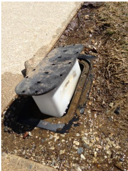
Figure 11: GKY sampler housing with sample container at FFG
