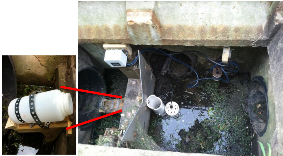
Figure 16: Bioinfiltration rain garden outlet structure and sampling equipment
