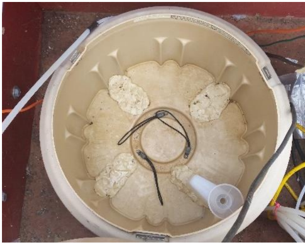
Figure 13: American Sigma autosampler housing for sample bottles.
