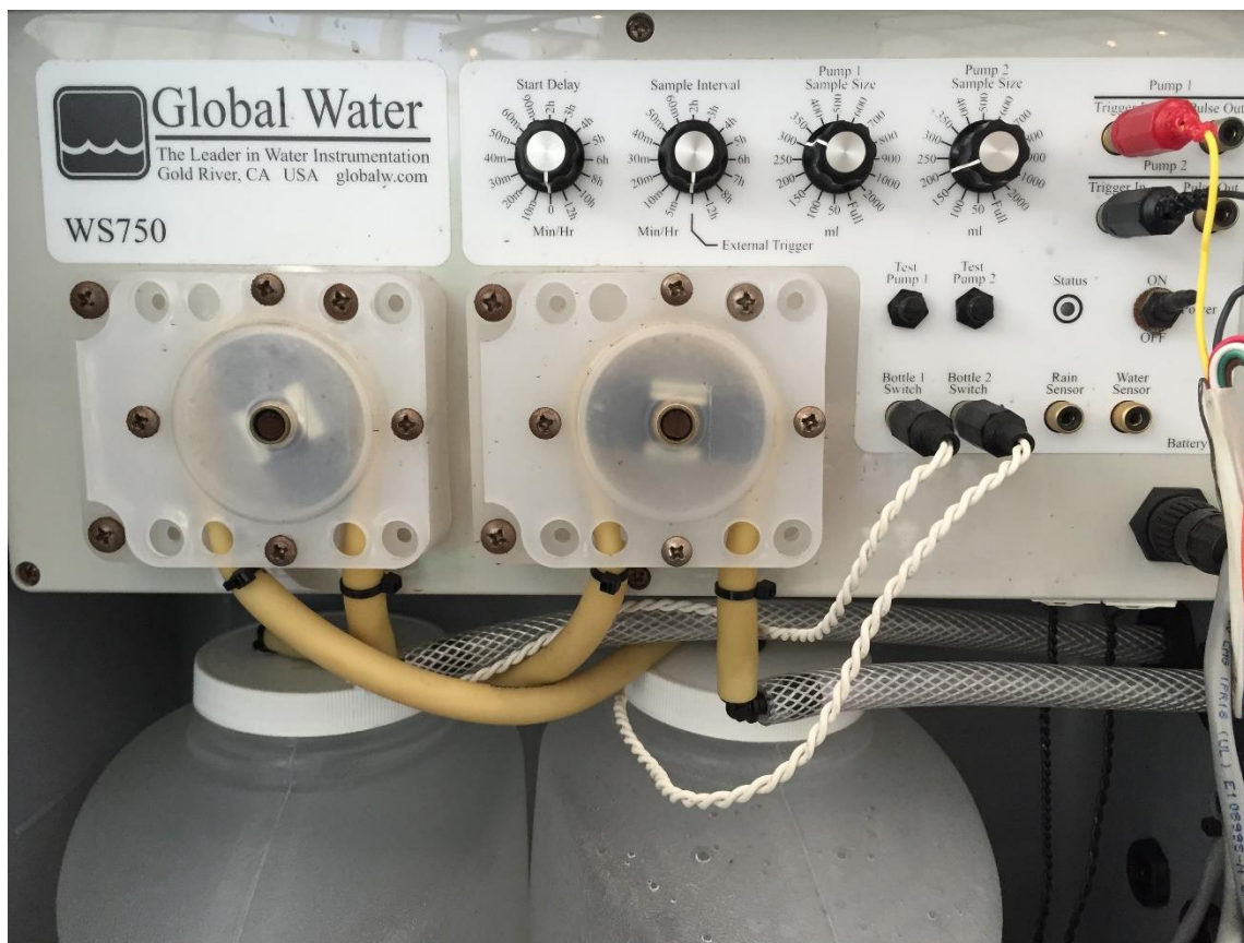
Figure 5: Global Water WS750 pump configuration and control panel.
