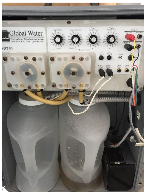
Figure 4: Global Water VS750 sampler with sampling bottles in place. Bottle 1 containing sample is positioned on right, beside the battery
