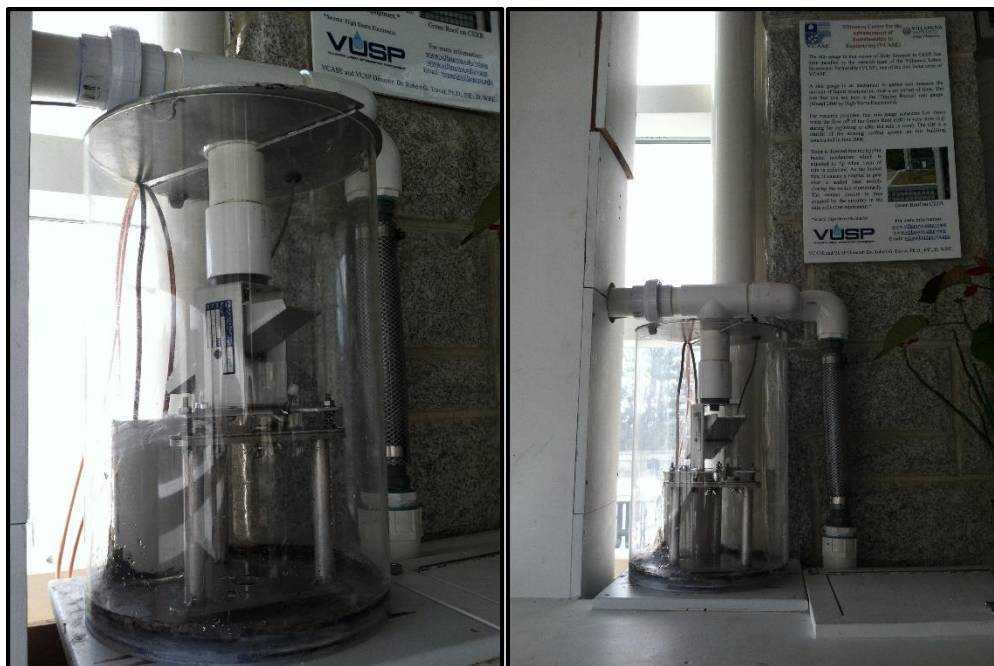
Figure 3: High Sierra Tipping bucket instrument in its housing; shown with PVC sample cup and copper pickup tubes for autosampler feed.
