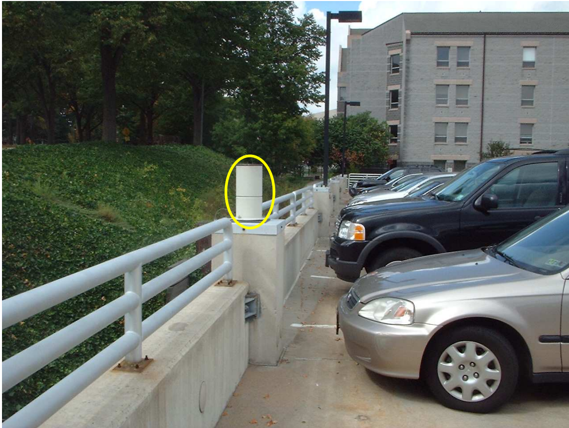
Figure 2-3: On site rain gage mounted on the edge of the parking deck.
