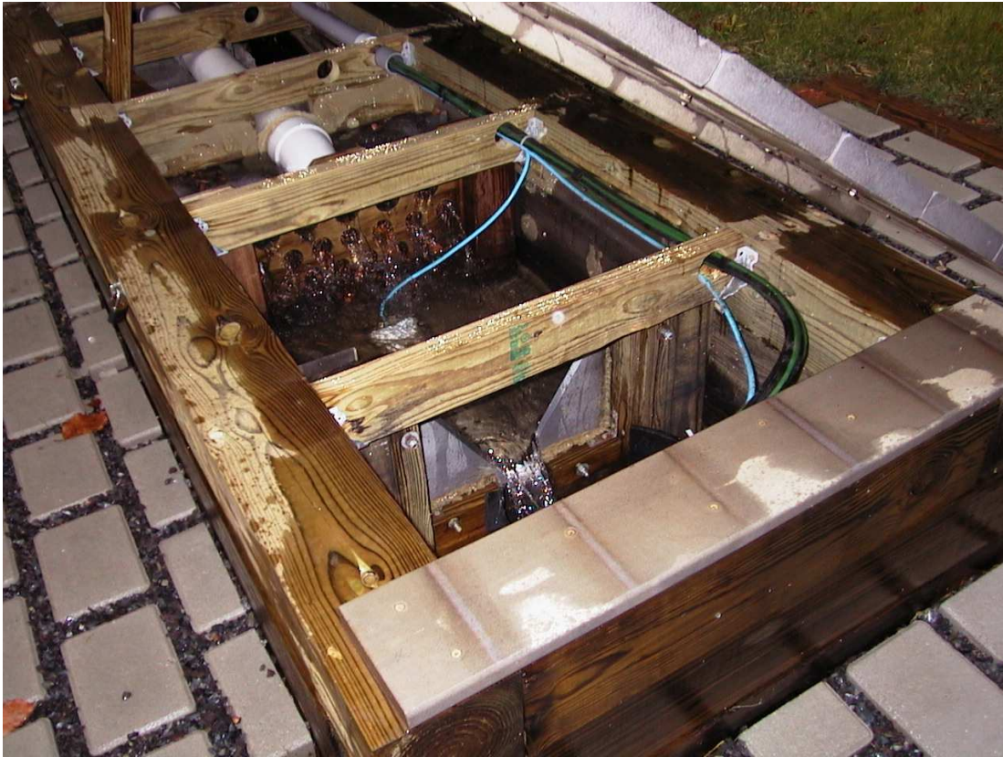
Figure 2-5: V-Notch Weir during a storm event.
