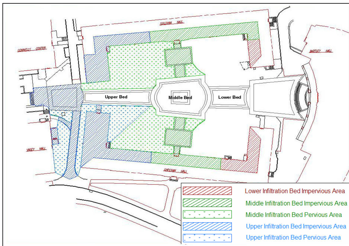
Figure 3. Drainage area schematic of the site
