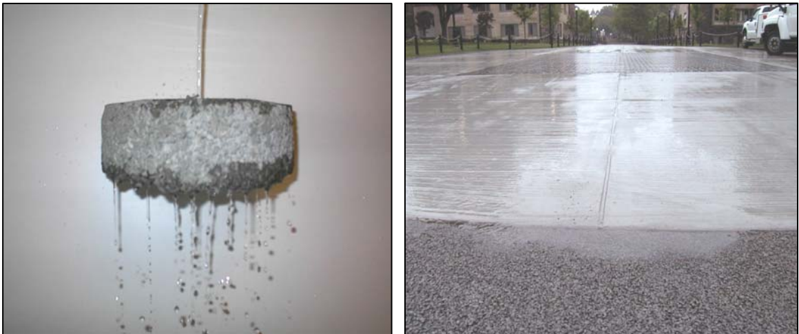
Figure 5. Illustration of the ability of porous concrete to convey water
