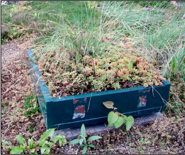
Figure 3.1. Villanova Weighing Lysimeter
