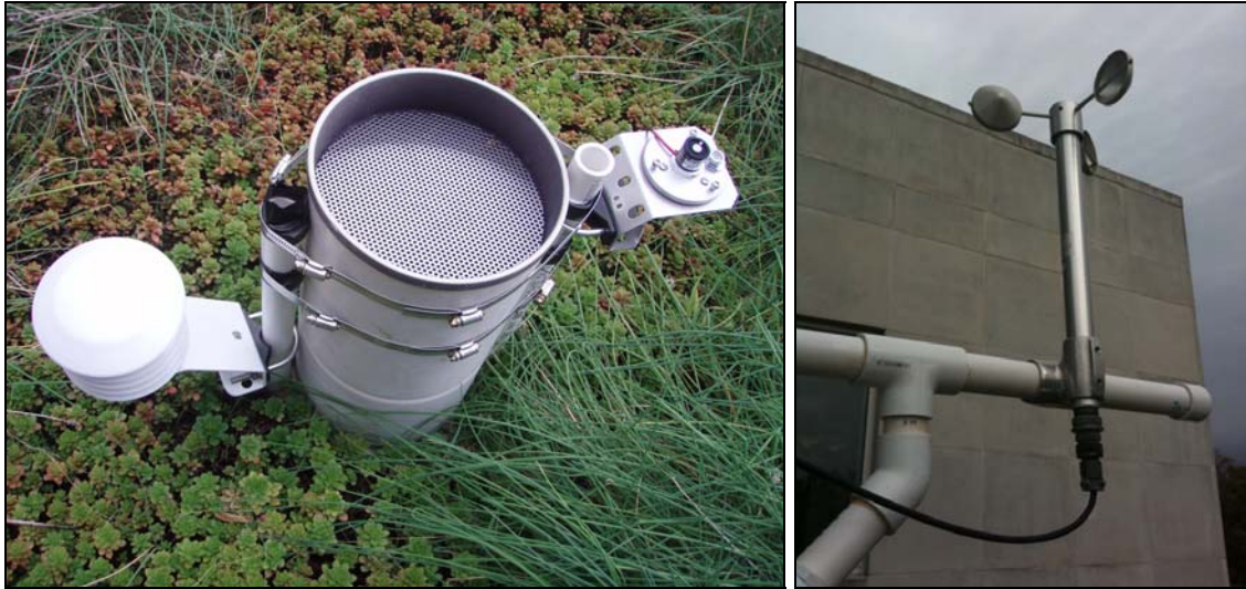
Figure 3.4. Villanova Green Roof Weather Station Including a Temperature and Relative Humidity Probe, Rain Gauge, and Pyranometer (left), and Anemometer (right).
