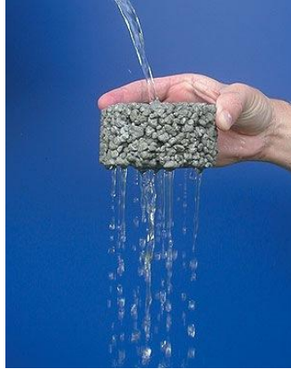
Figure 2.1: Water Traveling Through Pervious Concrete (Ziger and Snead 2007)
