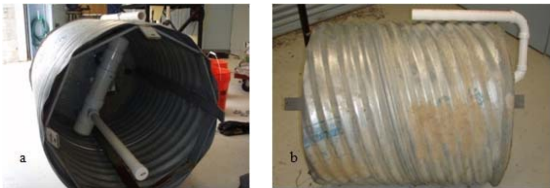
Figure 14 Bioretention Lysimeter Design with the top view (a) and side view (b).
