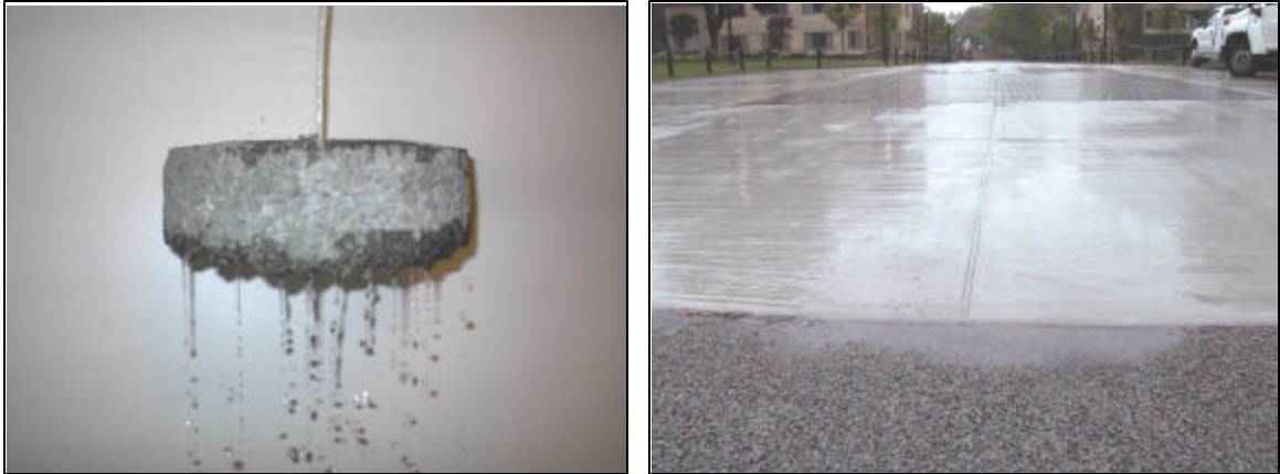
Figure 5. Illustration of the ability of porous concrete to convey water
