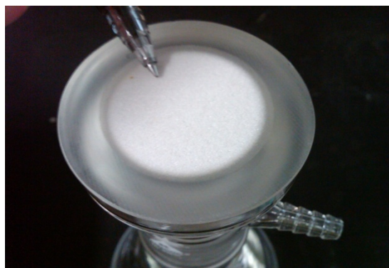
Figure 5-4 Top) Filter apparatus Bottom) Porous glass filter close up
