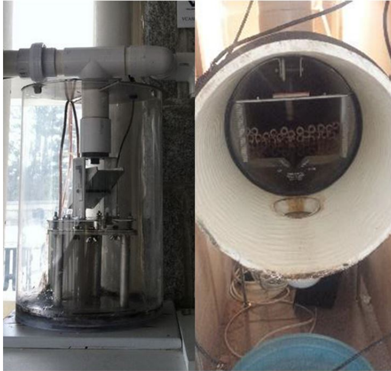
Figure 3.8: Metering Tipping Bucket (Left) and Thelmar weir (Right) Used for Overflow Measurements. (VUSP)
