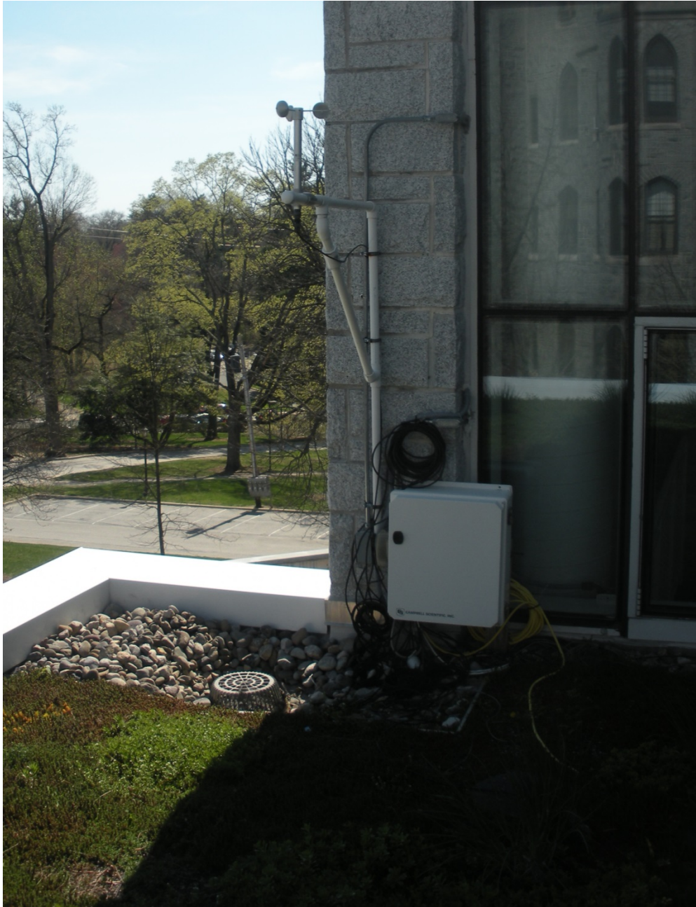
Figure 3.5: Location of Campbell Scientific Data Logger and Met-One Anemometer (VUSP)
