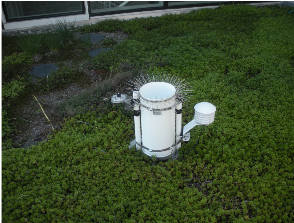
Figure 3.6: Site of Rain Gauge, Temperature, Relative Humidity, and Solar Radiation Instrumentation. (VUSP)
