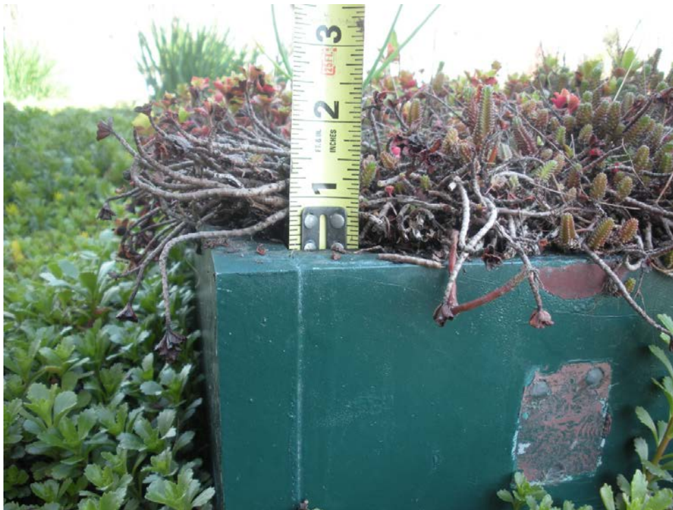
Figure 4.19: Photo of Lysimeter Showing Surface of Media below the Upper Lip of Sidewalls by approximately 6.5mm (0.25in)
